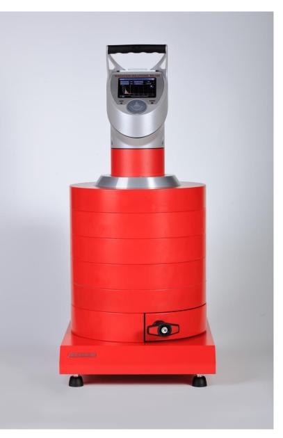
where one half is fixed to the base and the second one hangs on a hinge and serves as a door. Samples are situated in a measuring chamber behind the door. Size of the chamber is enough for samples with maximum volume around 350 ml. Detector or spectrometer is inserted in a central hole in the rings. A lock constructed in the second ring defines the detector position.
